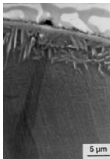
Fig. 7 Scanning electron micrograph of cross-section image of etched spheroidized Ti-6Al-4V. This same particle was used for analysis, the results of which are in Fig. 6 (analysis line in the lower part of the picture).
